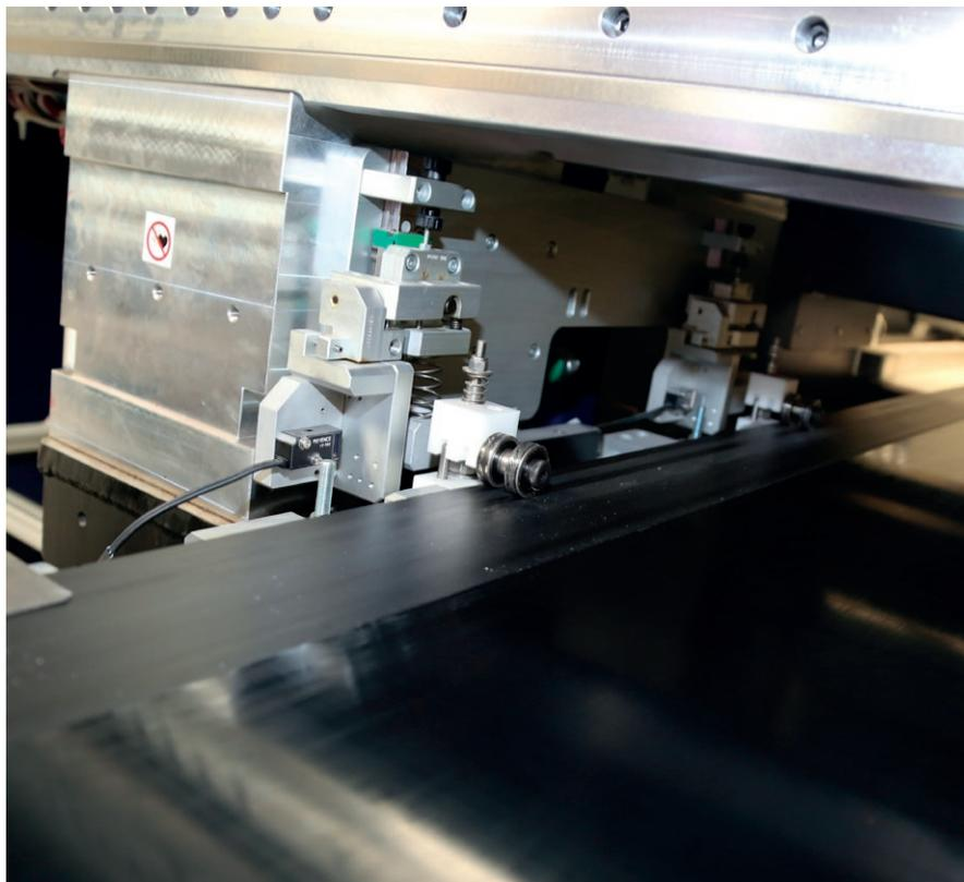
**Head crash protective system by 2 laser-beam sensors.** It allows the precise detection of the printing media unevenness by preventing the contact with the printing heads.
