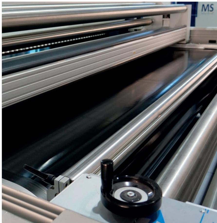
**Heated driven pressure roll.** Mechanical cylinder, electrically heated, that stretches the fabric on the printing belt in an optimal way.
